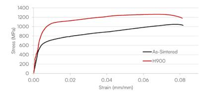
All data represents samples with 15 mm printed and 13 mm sintered thickness, sintered using a standard cycle in Rapidia's F2 Vacuum Furnace. Tensile testing, hardness and density measurements, and metallography were performed at an accredited third party laboratory. Corrosion resistance was determined in-house at Rapidia. Note that material performance is influenced by numerous factors such as print quality, furnace loading, and part thickness and geometry.
