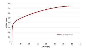
All data represents samples with ~10 mm printed and ~6 mm after machined thickness - sintered in around 12 hours using Rapidia's F2 Vacuum Furnace. All characterization was performed in-house at Rapidia. Values listed are the samples printed in the XY-plane. Values for samples printed along the Z-axis can be lower depending on print quality. Note that material performance is influenced by numerous factors such as print quality, furnace loading, and part thickness and geometry.
